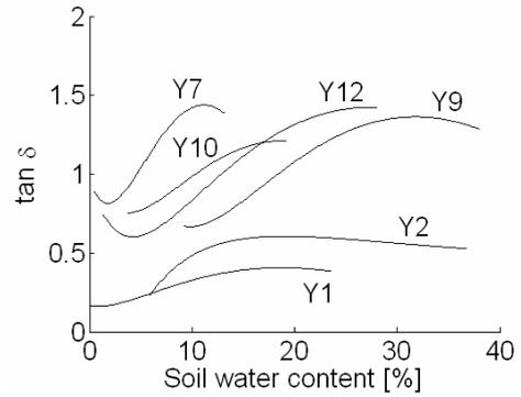
**Figure 3.** Loss tangent ( $\tan \delta$ ) versus soil moisture at six stations of the Murrumbidgee network in Spring 2006. Curves were generated from best-fit polynomial equations for each soil.
