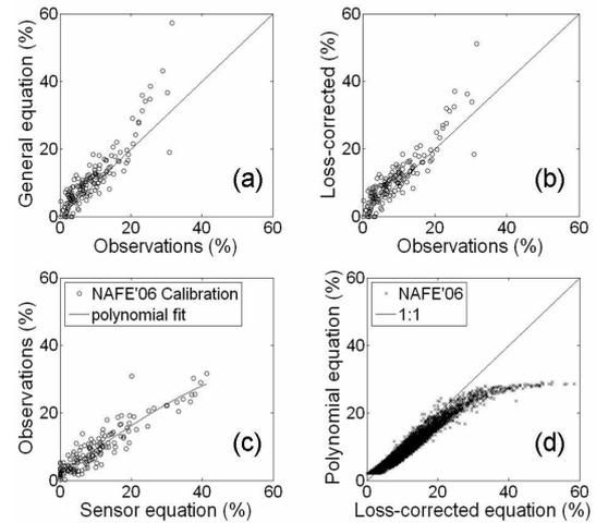
**Figure 5.** Different calibration equations: in a) the general equation; in b) the loss-corrected equation; in c) the polynomial equation. In d), the polynomial equation is plotted against the loss-corrected equation with the whole NAFE'06 data set.
