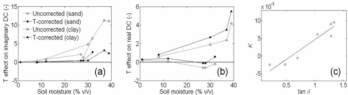
**Figure 1.** Temperature effect on the uncorrected DC and the DC corrected for temperature effect by the manufacturer's algorithm: a) the imaginary component of DC; b) the real component of DC. With clay, the observed temperature effect on real DC is increased by the manufacturer's correction. In (c), the temperature effect ( $K$ ) for a 15°C increase is shown as a function of loss tangent.
