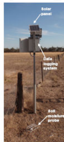
Fig. 4. Set up of a typical semi-permanent station
