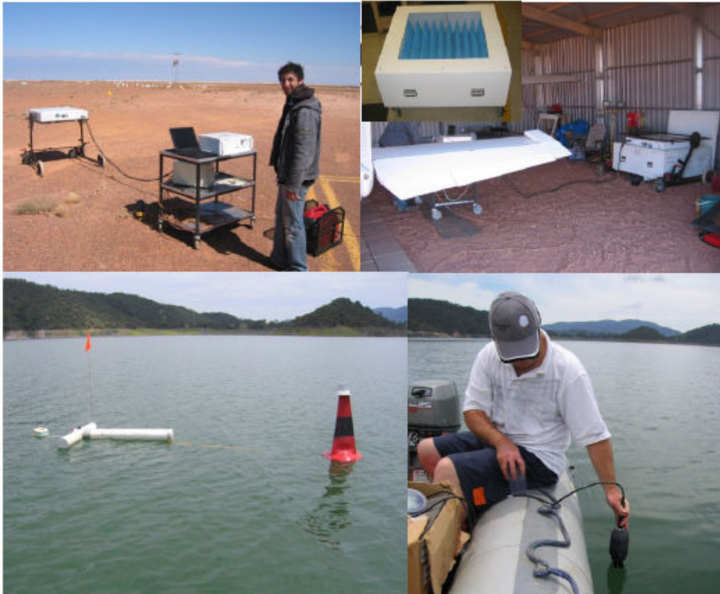
Figure 5-9. Upper left: undertaking a sky cold point calibration with PLMR; upper right: undertaking a warm point calibration with the calibration box shown in the inset; lower left: the buoy used to monitor water temperature and salinity; lower right: undertaking a boat transect of water salinity and temperature.
