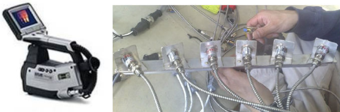
Figure 3-4. Thermal imager (left) without the 80° FOV lens attached and thermal infrared radiometers (right).
