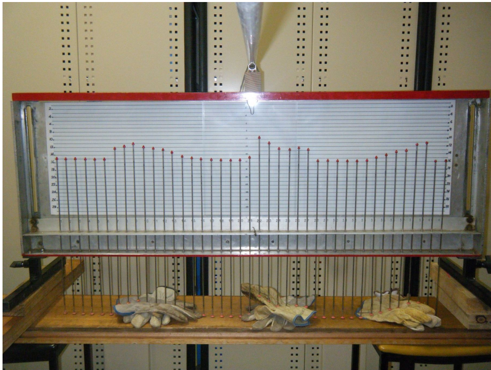
Figure 7-3. Pin profiler for surface roughness measurements.
