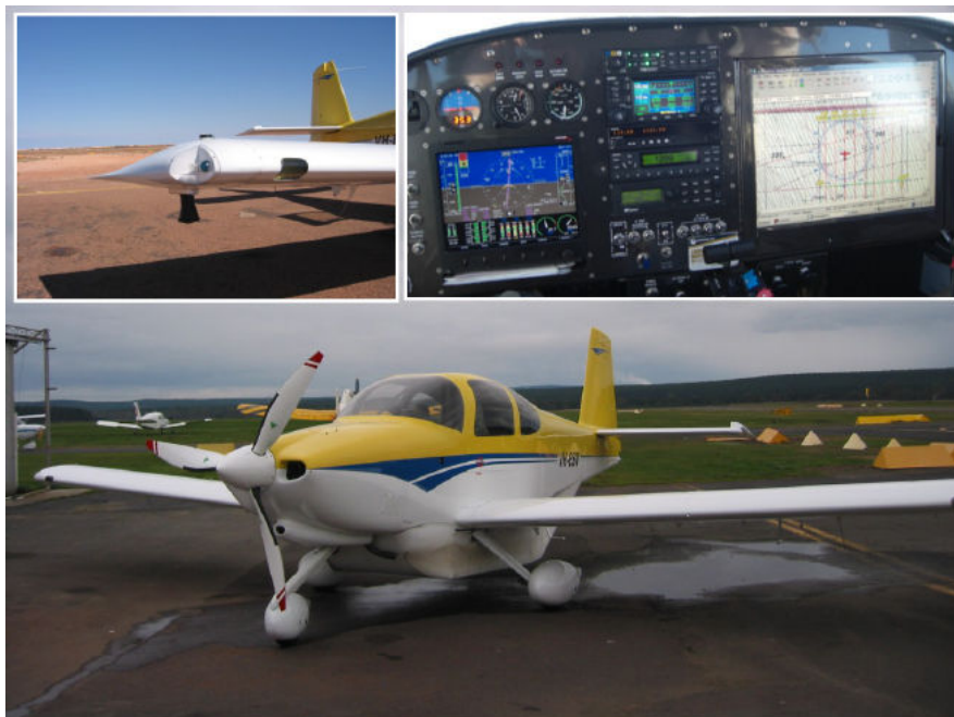
Figure 3-1. Experimental aircraft showing a wingtip installation in the left inset, and the cockpit with cockpit computer display in the right inset.
