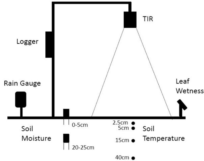
Figure 6-1. Schematic of the temporary monitoring station.
