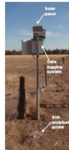
Fig. 4. Set up of a typical semi-permanent station
