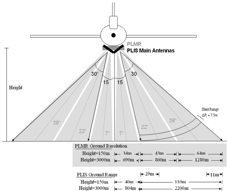
Figure 5-1. PLMR and PLIS viewing configuration on the RV-10 aircraft.
