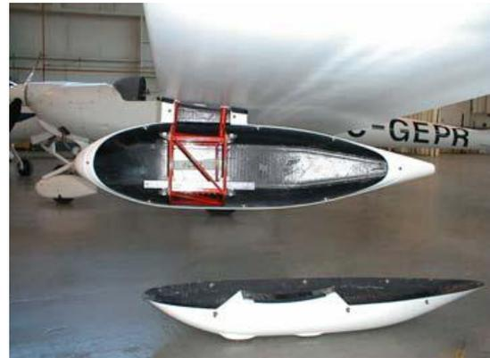
Figure 3-3. Experimental EOS aircraft showing the cockpit and the underwing pod.
