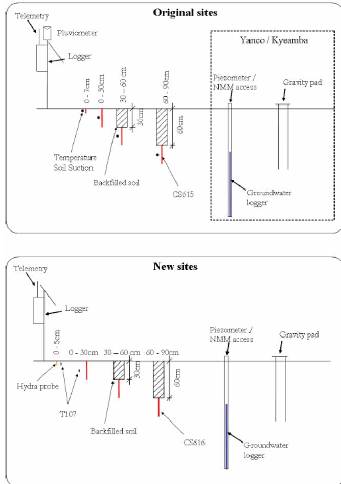
**Figure 4-5. Typical equipment at the original (2001) and new (2004) soil moisture sites in the Murrumbidgee catchment. Each site provides continuous data of rainfall, soil moisture at 0- 5cm (or 0-7cm), 0-30cm, 30-60cm and 60-90cm and soil temperature and accommodates periodic measurements of gravity, groundwater and TDR soil moisture measurements.**
