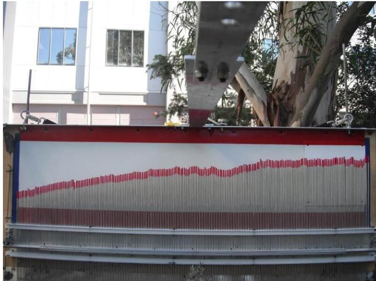
**Figure 7-5. Pin profiler for surface roughness measurements.**
