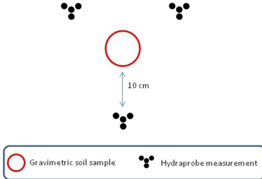
**Figure 6-10. A minimum of three Hydraprobe measurements should be made in a radius of 10cm around the gravimetric soil sample.**
