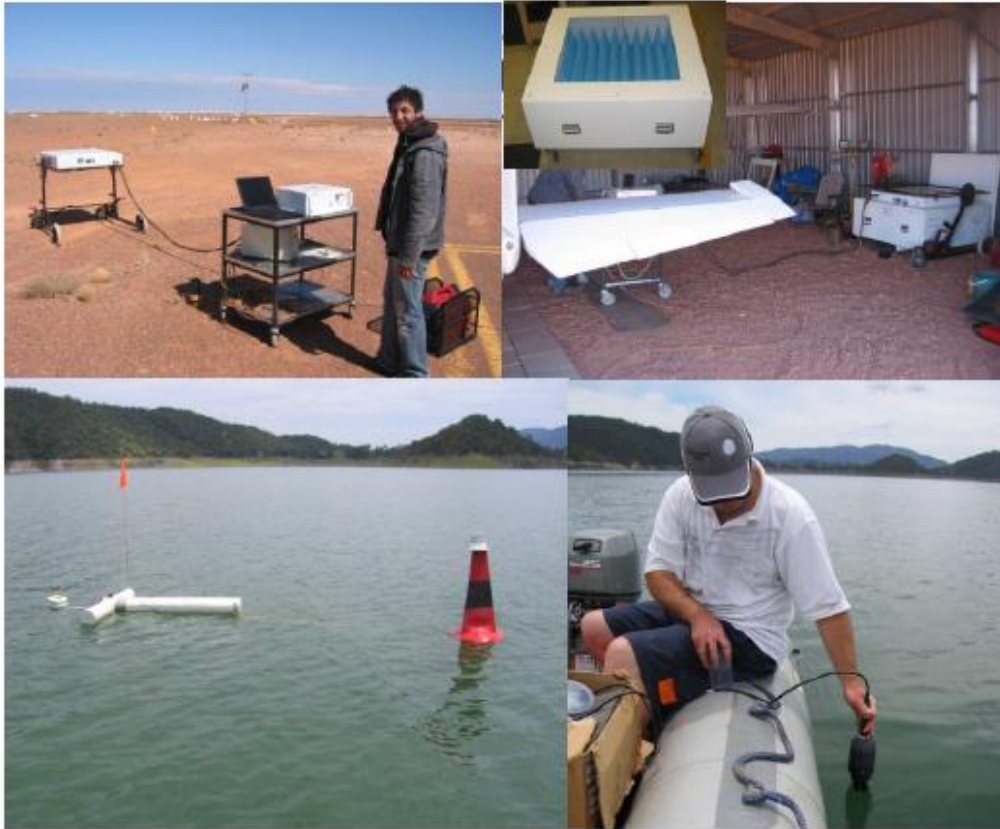
Figure 5-11. Upper left: undertaking a sky cold point calibration with PLMR; upper right: undertaking a warm point calibration with the calibration box shown in the inset; lower left: the buoy used to monitor water temperature and salinity; lower right: undertaking a boat transect of water salinity and temperature.
