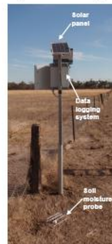
Fig. 4. Set up of a typical semi-permanent station
