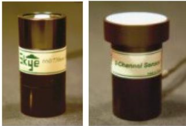
Figure 3-5. Multi-spectral sensors; downward looking sensor without the field of view collar attached (left) and upward looking sensor with cosine diffuser fitted (right).
